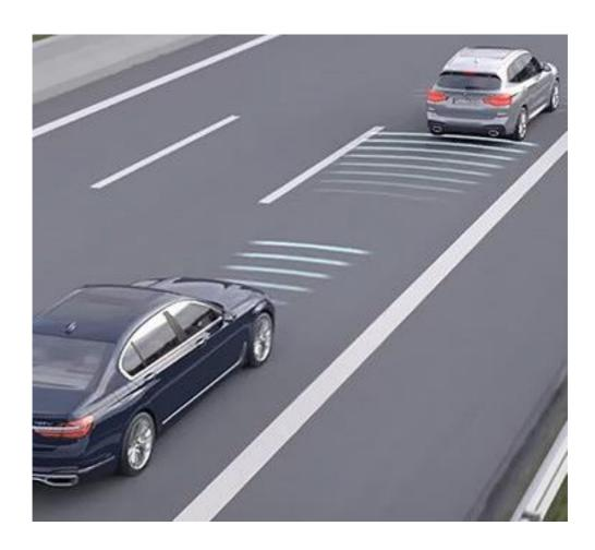
This cruise system enables you to keep a proper distance from the vehicle in front by constantly monitoring and adapting to its speed. These enhancements allow for more dynamic acceleration of your vehicle after stopping.
