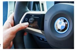
The **Assisted Driving Mode** combines **Distance Control** and **Steering Assistant** which supports the driver by actively centering the vehicle in the lane, maintaining speed, and keeping distance to the vehicle ahead.
