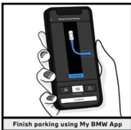
After the vehicle detects a parking spot or is near a recorded path, it will offer a maneuver. Engage the parking brake, exit the vehicle, and complete the maneuver by following the instructions in the My BMW App. Additionally, Remote Control Parking can be used to leave parking spots.
