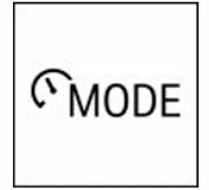
To activate Highway Assistant/Assisted Driving Plus, press the "I/O" button on the steering wheel and then the "Mode" button until you have selected Assisted Driving. Once all functional requirements for Assisted Driving Plus are met and "ASSIST PLUS READY" is displayed in the instrument cluster, confirm by pressing twice the "Mode" button again to activate the Highway Assistant.
