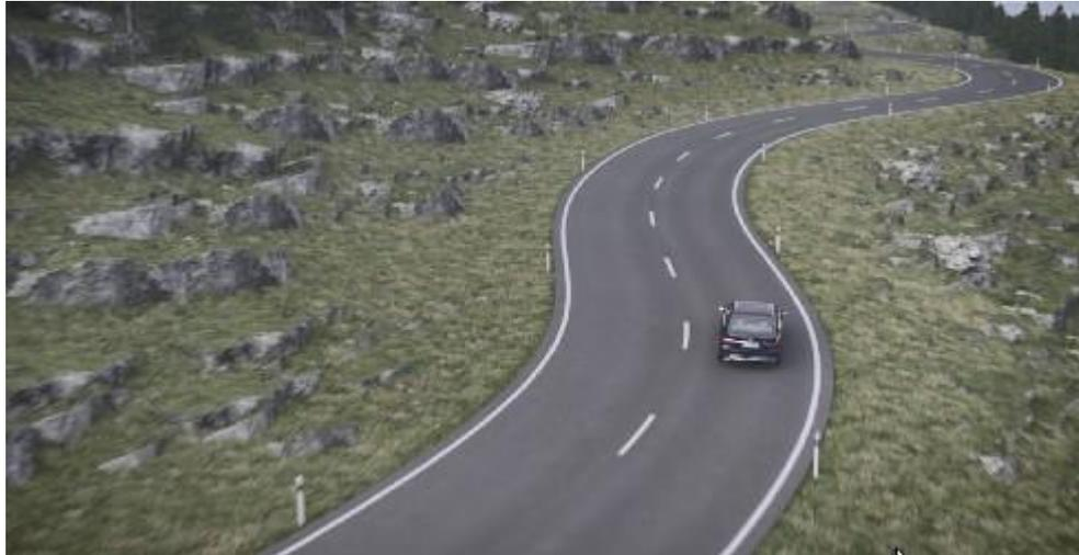
The Dangerous Curve Alert warns about upcoming, sharp or steep curves by sending a notification to the instrument cluster. The alert works with the Q4 2018 version (or later) GPS map.
